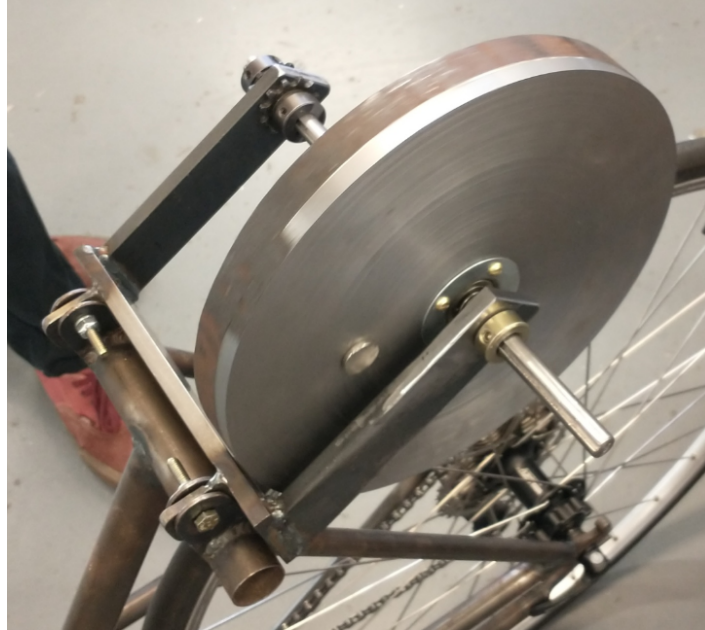
Figure 2: Mounting System and Flywheel
