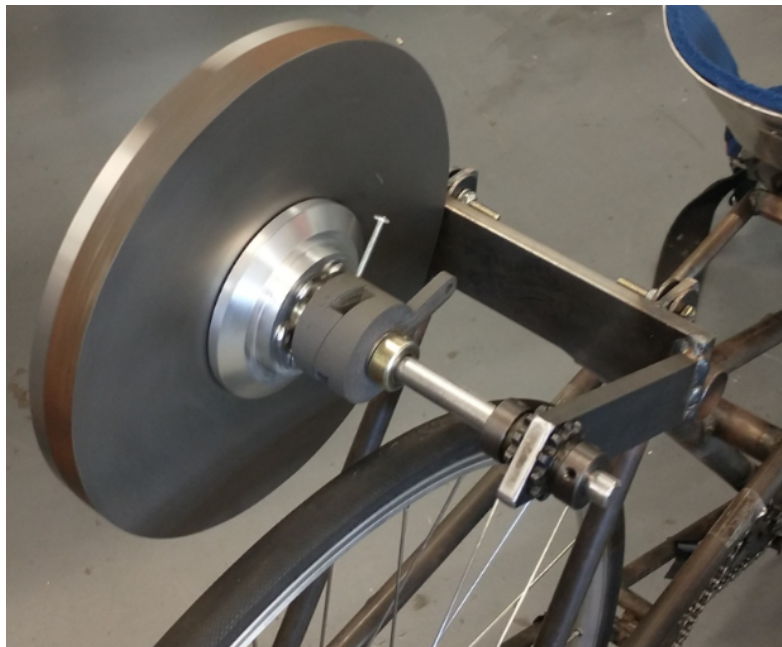
Figure 3: Energy Recovery and Storage System Assembly
